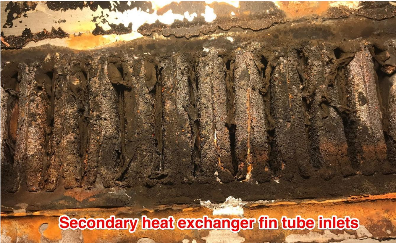
**Image 6** – Plugged and blocked tube inlets from corrosion and delaminated polypropylene liners.
